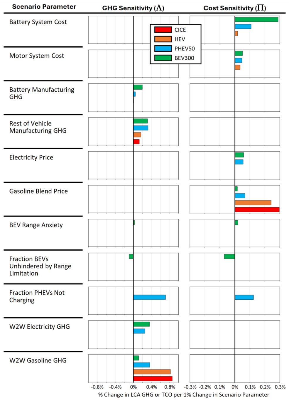
Figure 6. Sensitivity of Normalized LCA GHG and TCO to perturbations in scenario parameters.
